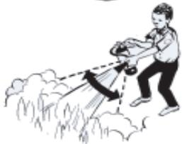
**S**weep the nozzle back and forth at the base of the fire.
