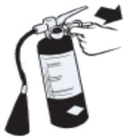
**P**ull the pin at the top of the extinguisher.
