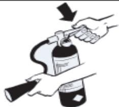
**S**queeze the handle to discharge the extinguisher (stand approximately 2.5 m [8 ft] away).
